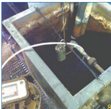
YSI sonde deployed at a metal coating/metal anodizing industrial waste pretreatment site.
